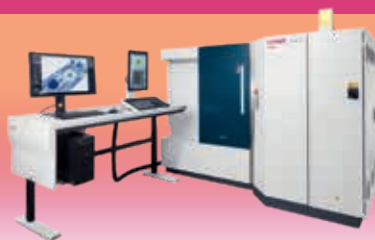
Comet Yxlon FF35 CT High Resolution Industrial Computed Tomography
